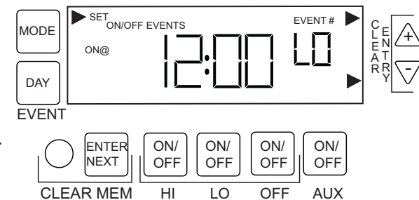
Figure 7 Setting the LO speed pump ON event
